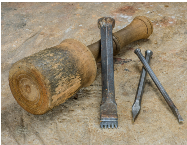
Above: (left to right) a hammer, tooth chisel, point chisel & flat chisel used in stone carving.
